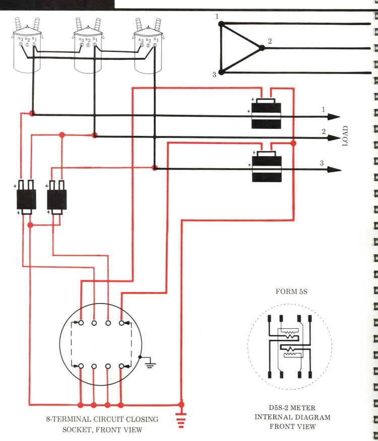
THE REGISTER MULTIPLIER EQUALS THE PRODUCT OF THE CT AND VT RATIO FOR SECONDARY-RATED METERS
