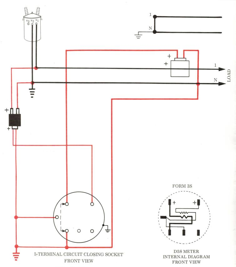
THE REGISTER MULTIPLIER EQUALS THE PRODUCT OF THE CT AND VT RATIOS FOR SECONDARY-RATED METERS
