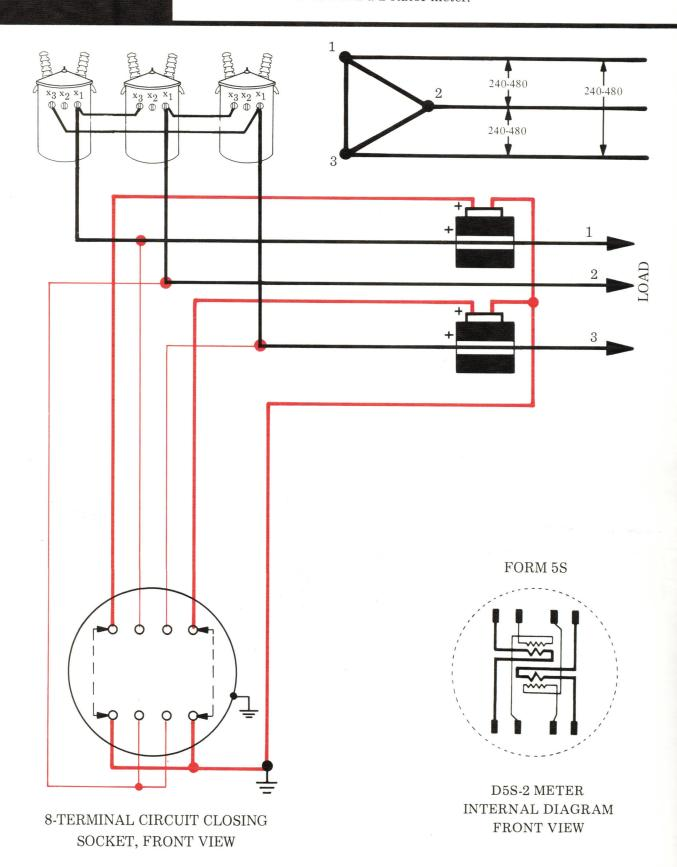
THE REGISTER MULTIPLIER EQUALS CT RATIO FOR SECONDARY-RATED METERS
